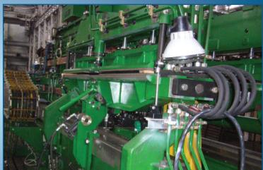
Machine is designed for resistance seam welding by direct current with crushing strip edges made from low carbon and low alloyed steels with carbon content up to 0,35% and electric (dynamo) steels with silicon content up
