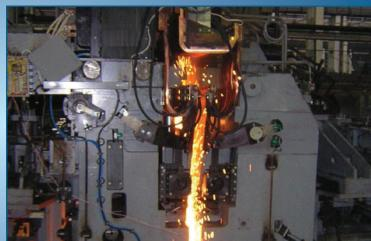
Using continuous processes in metallurgical aggregates in cold rolling workshops allows increasing performance of these aggregates and quality of production. Continuous process is provided by installation of welding machines for strips ends at the head part of aggregates. Width of welded strips from 700 mm up to 2 350 mm, thickness of welded strips from 1,2 mm up to 8,0 mm, max. strips section
