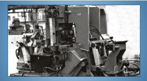
Machine KCO-32.01M is installed in the head part of tube mill and designed for FBW of strips ends ensuring continuous technological process pipes welding.
