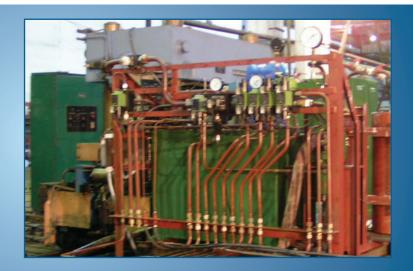
Machine MCO-100.01 (K-607) is designed for FBW of both straight and ring items with diameter from 500 mm up to 2 000 mm from aluminum, magnesium and titanium alloys, heat resistant and stainless steels of section up to 4 000 mm<sup>2</sup>. It is possible to weld cathode steel rods (blooms)
