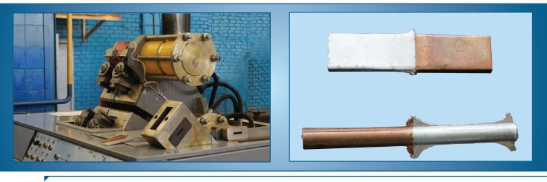
Machine MCXC-120,03M is designed for butt cold welding of round copper wire of grade MM as per GOST 2112-79; copper rectangular wire of grade ПMM; copper strip of grade AMM and copper bus bars as per GOST 433-78; copper rods of grade M1 as per GOST 1535-71; aluminum round wire of grades ПАТ, ПАМ as per TY16-705.451-87; aluminum rods of grades AQO, AQ1, AQ as per
