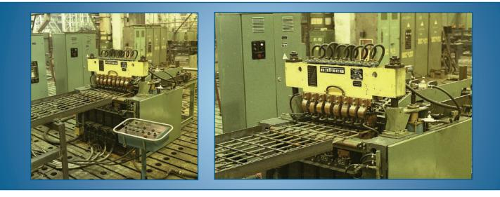
Machine MTM-207-1 is designed for multiple electrodes of reinforcing steel of grades of hardness AI, AII, AIII, BI. resistance spot welding of plane reinforcing nets from rods
