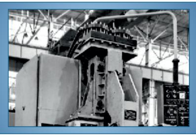
Machine MP are designed for projection welding of rim with rib during car brake shoes manufacturing.
