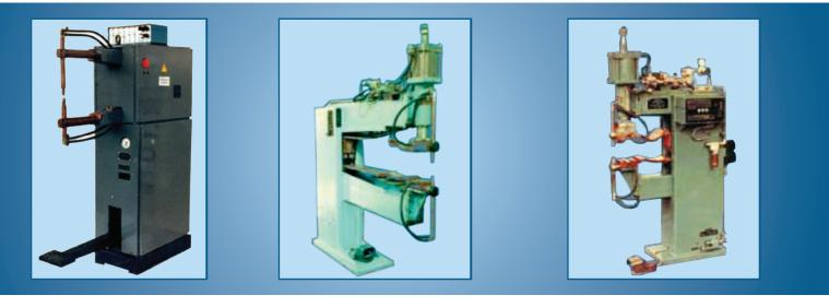
Machines MT are designed for resistance spot welding of parts from low carbon and stainless steels, cruciform joints of steel rods.
