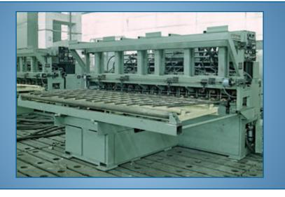
Machine MTM-32 is designed for multiple electrodes resistance spot welding of heavy reinforcing nets of wide range.
