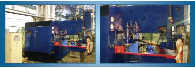
Machine MШB-80.01 is designed for step seaming welding by direct current with pressure tight and firm seam of light and titanium alloys, non-ferrous metals, heat resistant, stainless and low carbon steels.
