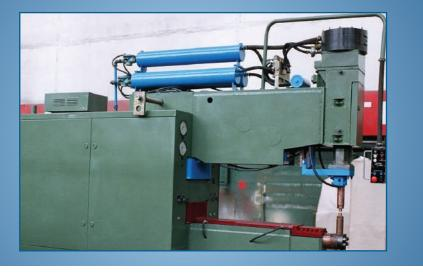
Machine MTB-80.02-1 is designed for spot welding by direct (rectified) current of various parts, including large ones, super duty products such as shell rings, trusses and other supporting structures. Maximum dimensions of welded parts are determined by electrodes stick-out, span of welding contour and upper electrode stroke.
