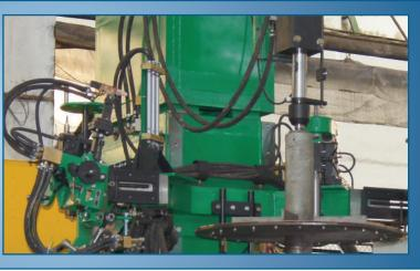
Automated device  $A\Delta\Gamma$ -507 is designed for arc welding of armature windings by tungsten electrode in inert gases.
