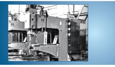
Machine MTB-100.01 is designed for spot welding by direct current of large super duty parts from aluminum, titanium and copper alloys, heat resistant, stainless and low carbon steels.
