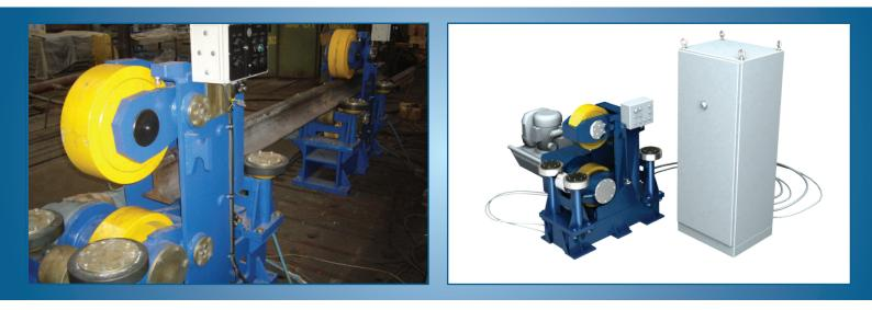
The pulling unit YT-02 is designed for transportation of continuously welded rails along the technological line of the rail welding plant to the pulling transporter. When the unit operates, the rolling sections drives are switched off ensuring electricity saving. The unit has a variablefrequency drive providing smooth changing of continuously welded rail traverse speed.
