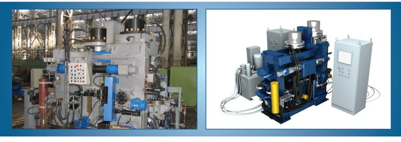
The welding machine of rails MCP-63.01A is designed for FBW of rails by continuous or pulsating flashing in stationary plant conditions. The machine provides rail alignment before welding according to the rail axis and to the height of the rail head, welds rails according to the preset program, removes weld flash around the entire contour of the joint after welding.
