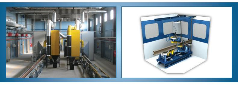
The rough grinding station  $\Pi\Gamma$ U-O1 is designed for abrasive treatment of the joint around the whole perimeter at the same level with the main profile along the rail. The rough grinding station is a cabin, equipped with local inputexhaust ventilation. The set of the station includes grinding machines for lateral sides, foot and head of the rail.
