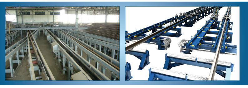
The transporter-distributor of continuously welded rail TPII-01 is designed for redistribution of the continuously welded rails at loading on the rail-carrying train in the conditions of multiple-flow production. The transfer of the continuously welded rail from one flow to another is carried
