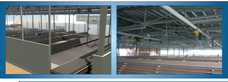
The storage area of the rail welding plant is designed for storage of the rails after offloading them from the supplier's transport and for subsequent uninterrupted delivery to the technological welding lines.
