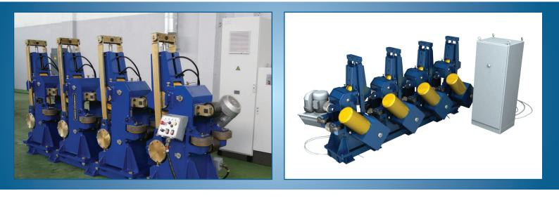
The modular pulling transporter TT is designed for operation as a part of technological line of the rail welding plant for transporting continuously welded rails.
