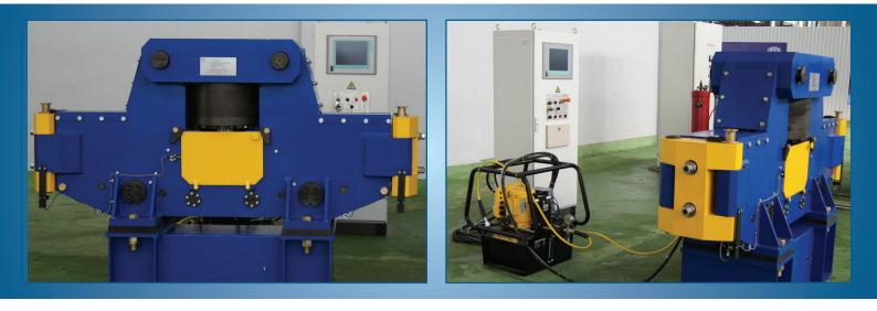
The special compact press  $\Pi$ MC-320 is designed for quality control of rail welded joints. It applies sampling method by means of testing check samples for static transversal bending.
