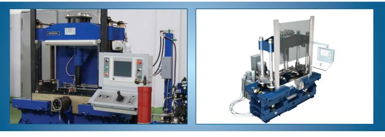
The cold joints straightening unit YIICX-01 is designed for straightening cold rail joints to meet the required geometry of the rolling surface and the rail head. The unit straightens the rail in horizontal and vertical planes on a base length of 1 300 mm and checking the rail bending on the length of 750 mm by laser sensors. Control system of the unit is based on an industrial computer. It allows recording and storing the dates of straightening process of the welded joint.
