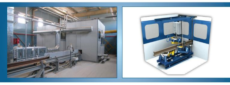
The rail final grinding station  $\Pi \Psi \square - 01$  is designed for final profile grinding of the welded joint of the rail head. The station is a cabin equipped with local input-exhaust ventilation. The set of station include grinding machine for final grinding of the rail head profile.
