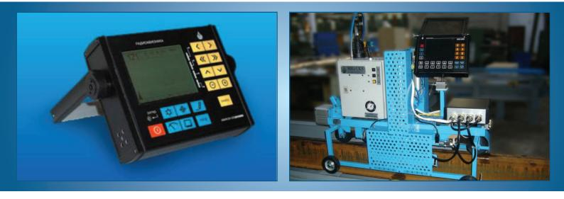
Ultrasonic defectoscope MI/IF-YKC is designed for testing the whole rail section (including blades of the rail foot) by means of 86 check channels. The ultrasonic testing system of joint allows detecting defects of various forms and orientations.
