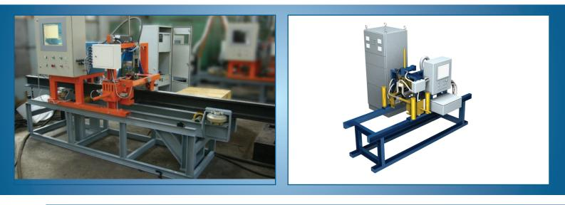
The high frequency inductive heating unit YHH is designed for differential heat treatment of rail welded joint. The control unit of the technological process ensures a complete automation of the process with min. participation of the operator and realizes the following functions:
